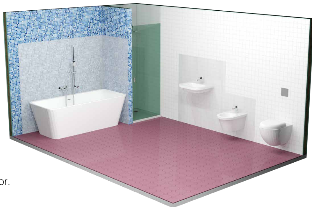
Fig. 37. Wall areas particularly exposed to water splashes in a bathroom (marked grey)
