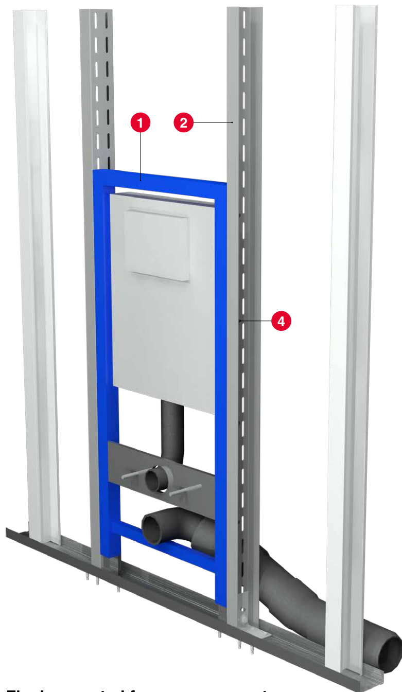
Sanitary flush-mounted frame in a partition wall
